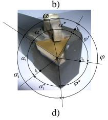
Fig. 5. Leftside scoring tool with coordinate traces to the location of the converter. a)-top view, b)-type front, c) - side view, d) - form an angle in front and above
